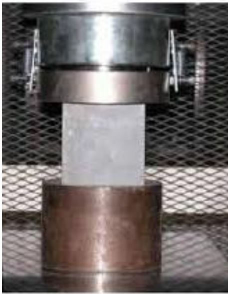
Fig. 1. Compressive strength test set-up
