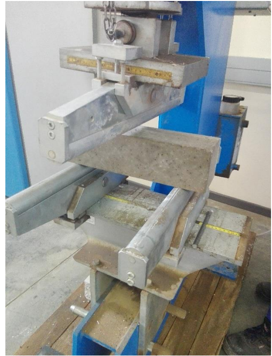
Fig. 3. Flexural strength test set-up
